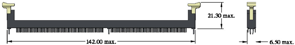
Figure 2 — Plated Through Hole (PTH) Connector Socket Outline
