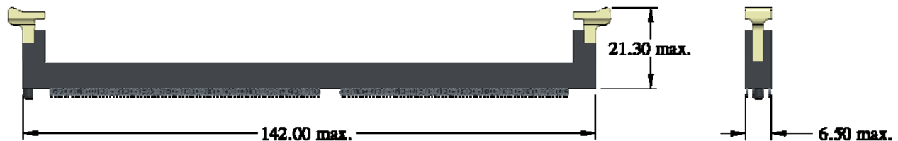
Figure 4 — Pressfit (PF) Connector Socket Outline
